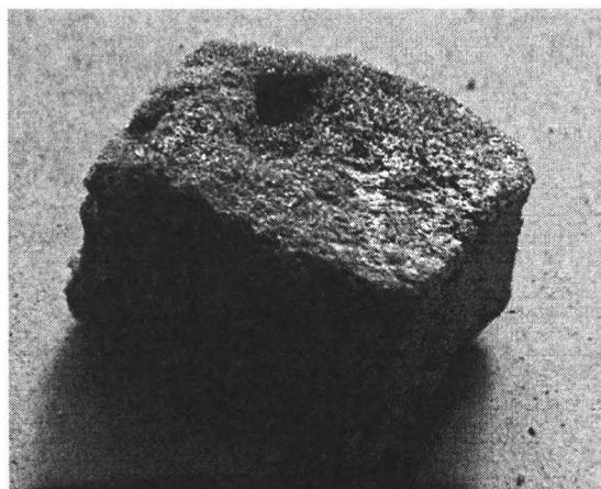
Fig. 5. PUF after termite-feeding test.
